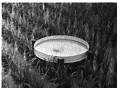
Fig. 1. Pan water trap set on a wooden stand at the crop level in paddy rice field.
