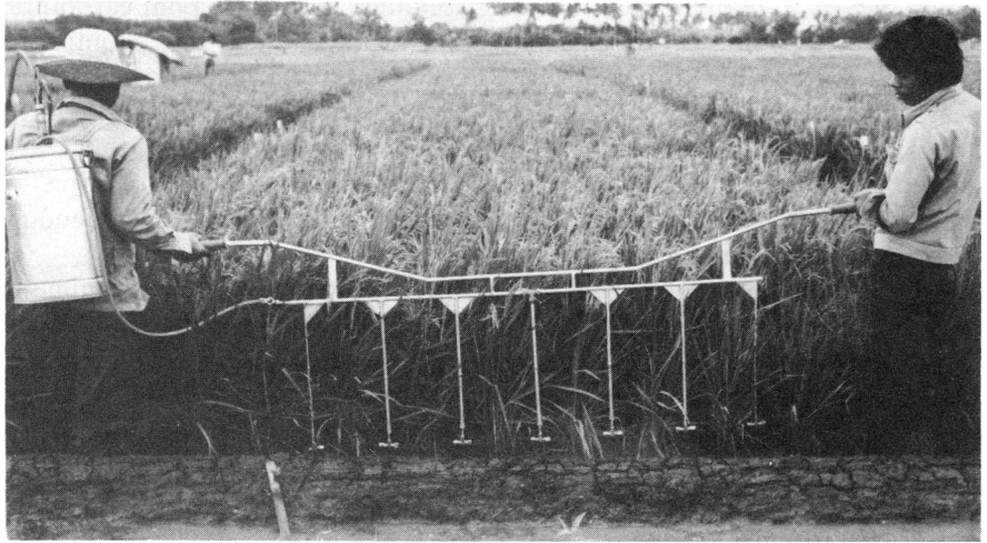
3. Six-row sprayer for applying insecticide to the base of the rice plants. IRRI, 1977.
