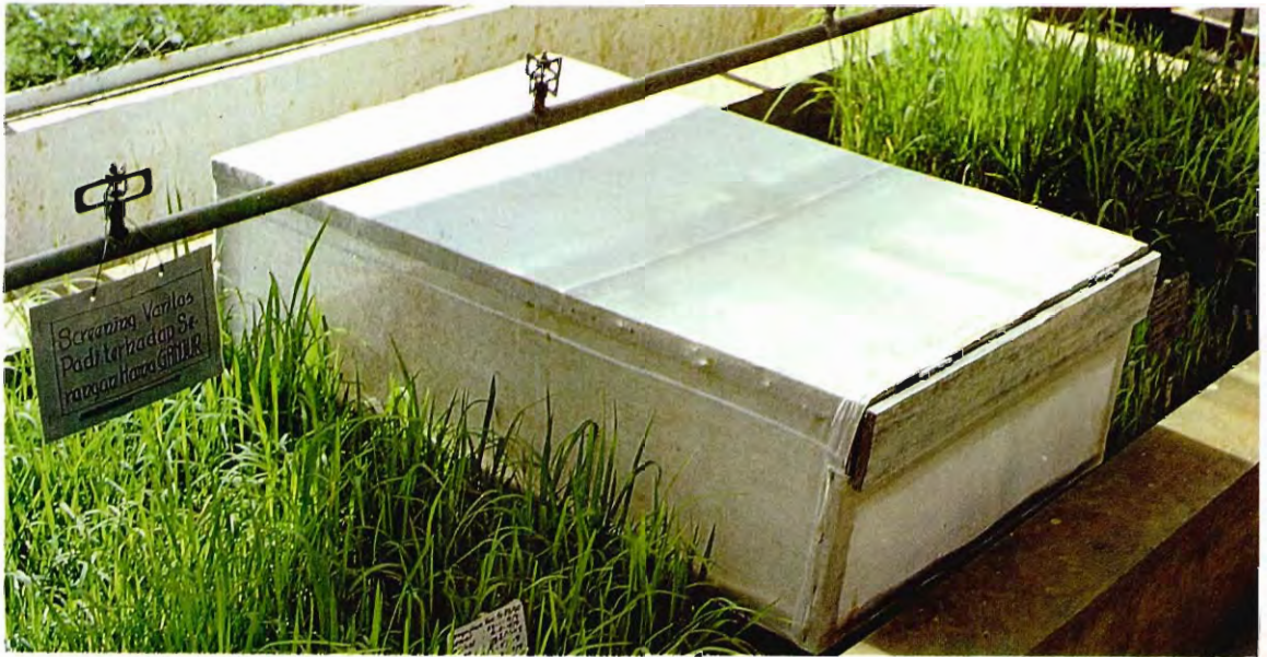
6. Nylon mesh cage used in infesting test plants with ovipositing gall midge adults.
