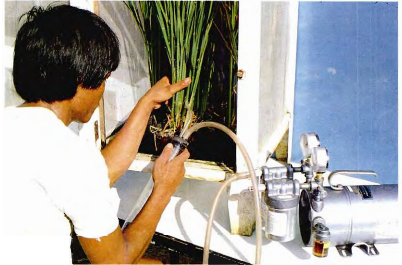
10. Suction machine for collecting hoppers.
