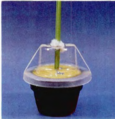
37. Left: apparatus used for the collection of honeydew with bromocresol green-treated filter paper. Right: blue spots produced by the honeydew of the brown planthopper on bromocresol green-treated filter paper and purple spots on a ninhydrin-treated filter paper.
