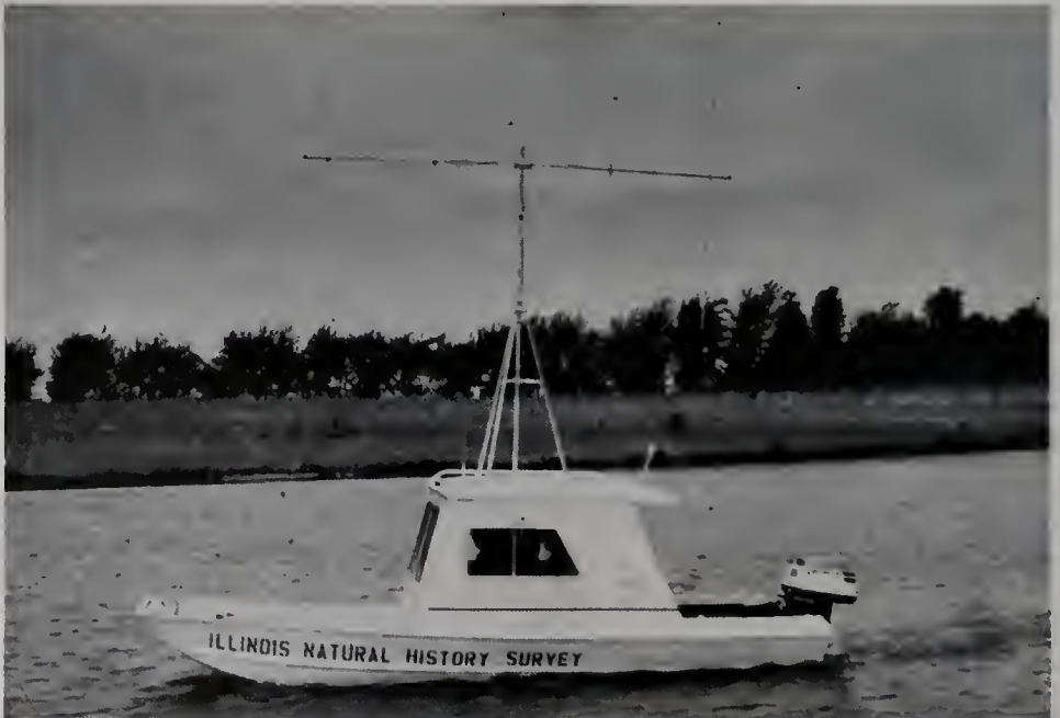
Radiotelemetry boat used for tracking and locating fish that had radio transmitters placed within their bodies.
