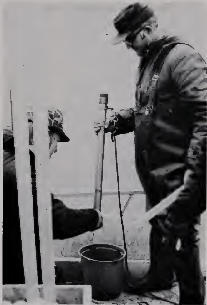
Taking sediment core samples from the Lake Sangchris basin for trace metal analyses.
