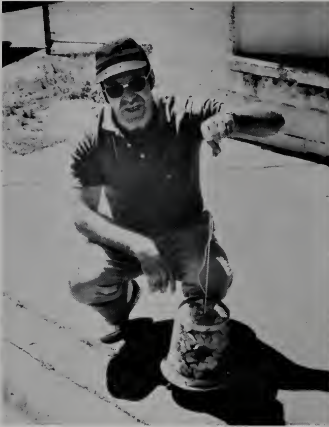
Artificial substrate sampler used in benthic studies at Lake Sangchris.
