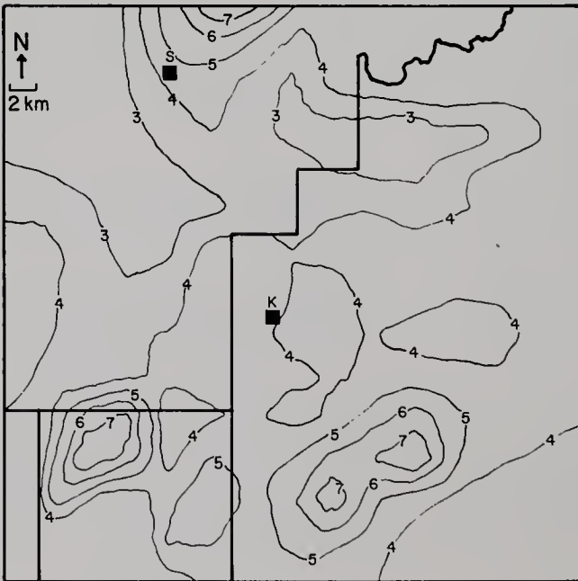
Fig. 6.—Distribution of cobalt ( \mu\text{g/g} ) in the soils surrounding the Kincaid Generating Station.
