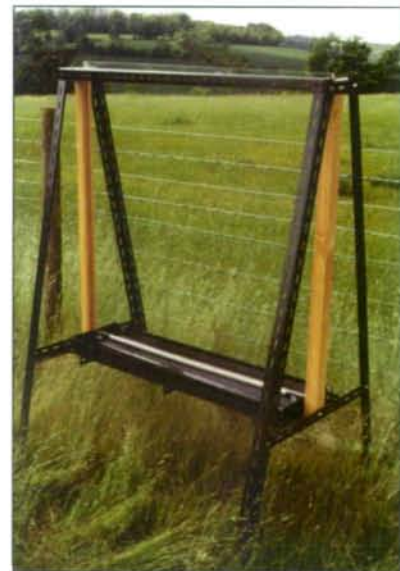
Fig. 9. Window trap. A perspex sheet (approximately 1x1m.) is mounted vertically on a metal frame. Flying insects are intercepted and fall down into fluid-filled collection troughs running along the base of the 'window'. Separate troughs on either side of the 'window' allow an assessment of numbers of insects moving in the two opposite directions.
