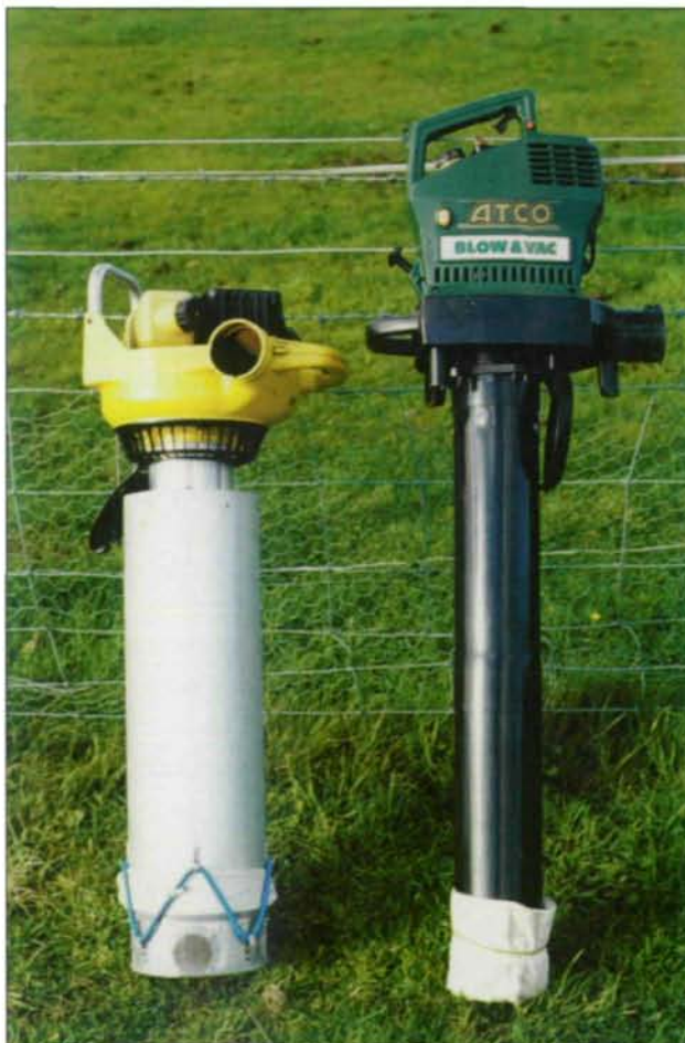
Fig. 2. Two types of G-Vac suction sampler. Right: the simplest design has a net collection bag inserted into the inlet tube and secured around the nozzle. The inlet tube has a cross-sectional area of 0.01m 2 . Left: alternative design where a custom-built inlet tube has a larger cross-sectional area (0.025m 2 ) and a flange with gauze-covered holes that is mounted beyond the collection bag to allow unimpeded entry of air into the inlet tube. Both samplers are powered by 30 cm 3 engines.
