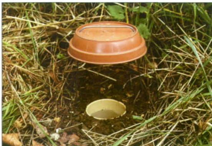
Fig. 7. Pitfall trap. A collection vessel (plastic, metal or glass, approximately 8-10cm. diameter) is embedded into the soil so that the rim is at or slightly below the soil surface. Epigeal invertebrates fall into the vessel which contains a small amount of preservation fluid. Rain-shields (in this case, an inverted plant pot saucer held in place by a metal wire frame) can be used to prevent the trap from flooding in wet weather.
