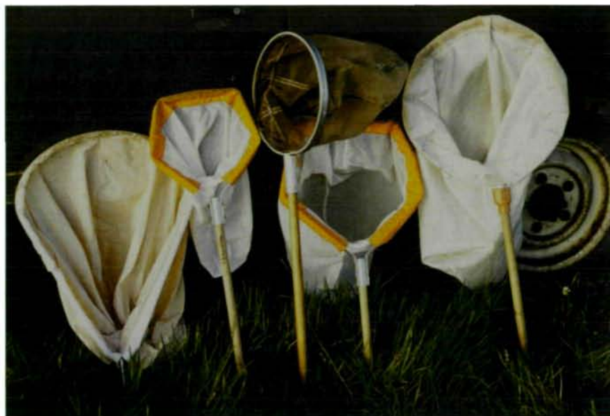
Fig. 5. Sweep nets. A range of sweep nets, illustrating the potential variation in size, shape and net material. The net in the centre is made with semi-rigid gauze netting designed to maintain the open net shape permanently.
