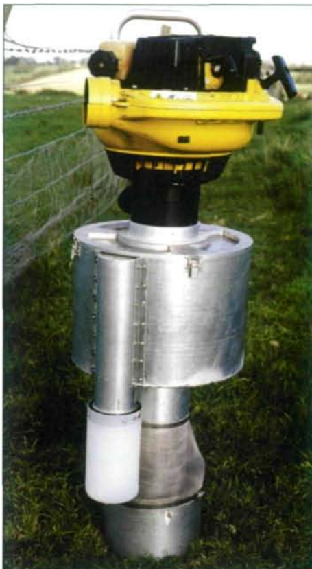
Fig. 3. Vortis suction sampler. Suction is provided by a 30 cm 3 engine (top). Air is sucked into the inlet tube through a gauze cone (bottom), drawn through a set of radiating internal vanes that generate a vortex and then into an expansion chamber (middle). Insects that are circulated by the vortex in the expansion chamber are propelled by centrifugal forces into an escape tube mounted on the side (middle left) and drop down into a detachable collection vessel below.
