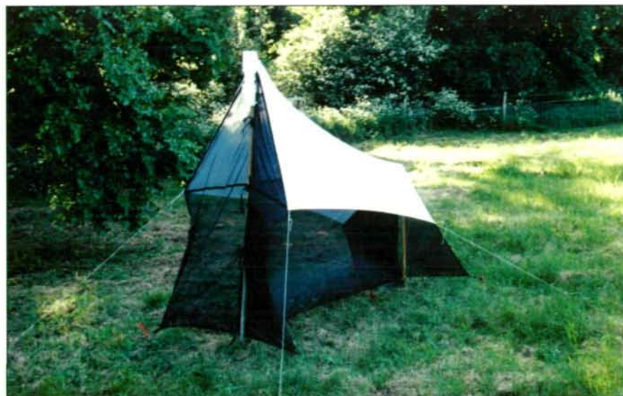
Fig. 10. Malaise trap. Vertically positioned sheets of black netting arranged like an open-sided tent intercept the movement of insects through the habitat. Once intercepted, insects respond phototactically and move upwards towards the white roof. The inclined ridge of the 'tent' funnels the insects towards the top corner, where an aperture leads into a collection vessel (top left) filled with preservation fluid.
