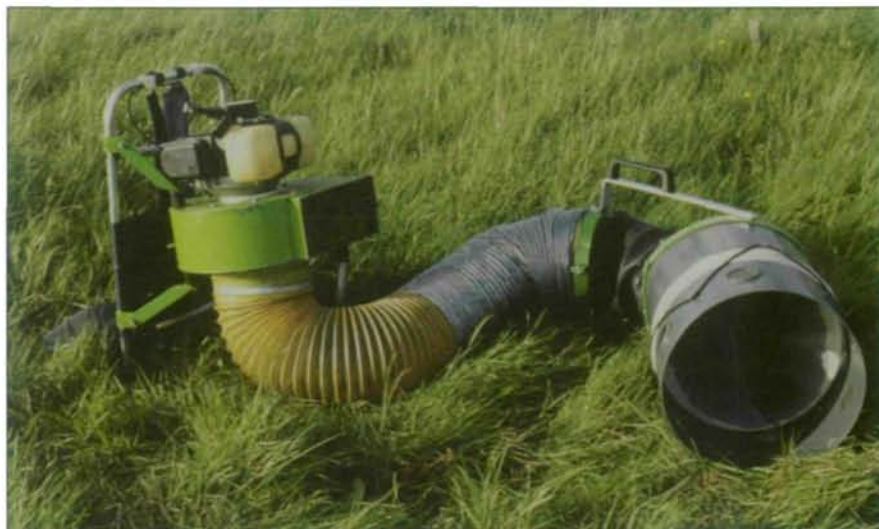
Fig. 1. D-Vac suction sampler. The engine and fan unit is mounted on a backpack frame (left) and connected via a long flexible hose (middle) to the inlet cylinder which contains the sample bag (right).
