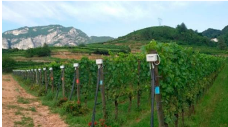
Figure 1: set-up of vibrational transducers in a vineyard from Mazzoni et al. (2019b)
