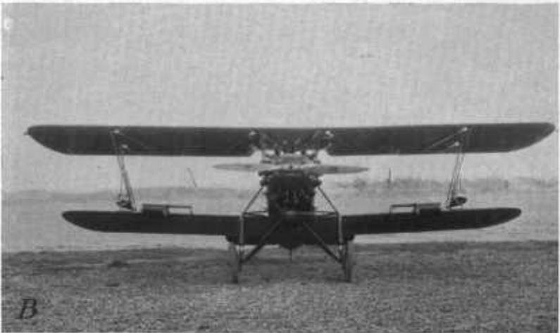
A , A single-compartment insect trap adapted for use on the leading edge of the lower wing of a biplane; B , a biplane equipped with two single-compartment insect traps.
