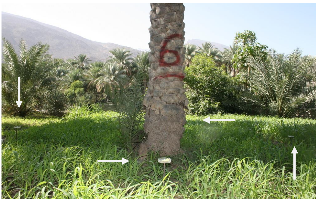
Figure 4.1 Distribution of WSP, 1.5 meter around Date Palm trunk in different directions (East, West, South and North).
