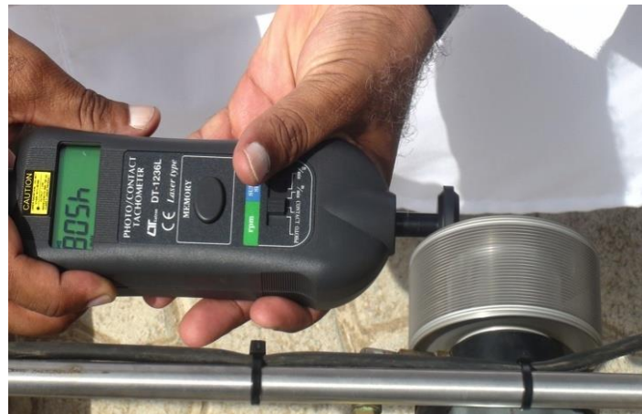
Figure 4.3 Adjusted RPM speed by digital tachometer.
