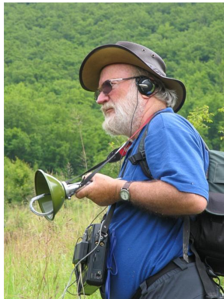
Fig. 6: Matija with a light version of the ultrasound detector with a microphone attached to a parabolic reflector (front light reflector of Renault 4) and Compact Flash Recorder during field work in Romania, June 2008 (photo: T. Trilar).
