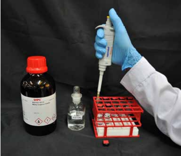
Fig. 11.2. Preparation of ME test solution using a micropipettor in a fume hood.
