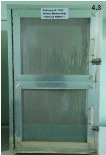
Fig. 4.3. Aluminum rearing/oviposition cage (56.5 cm × 56.5 cm × 91.5 cm) with aluminum wire mesh on three sides, top, and doors for ventilation.
