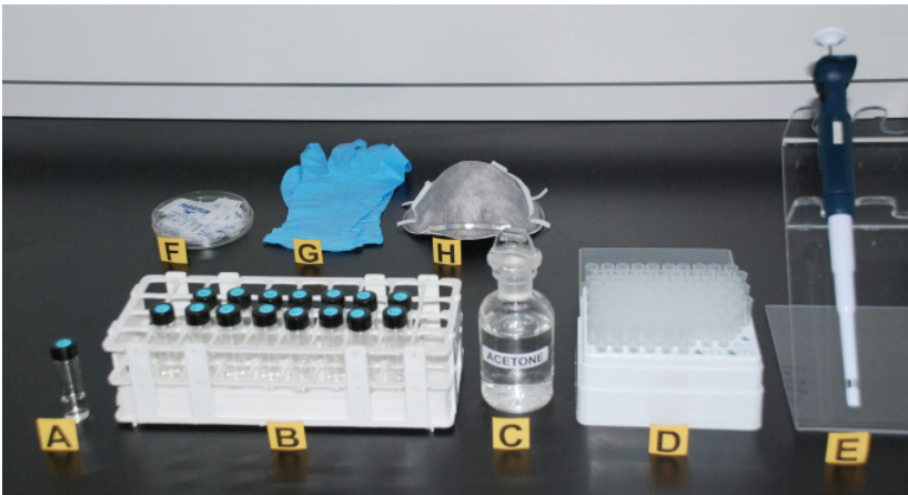
Fig. 5.2. Materials for preparation of serial dilutions: (A) stock solution, (B) 6-mL screw cap vials with label, (C) technical-grade acetone, (D) pipettor tips, (E) pipettor, (F) parafilm strips, (G) disposable nitrile gloves, (H) disposable mask.
