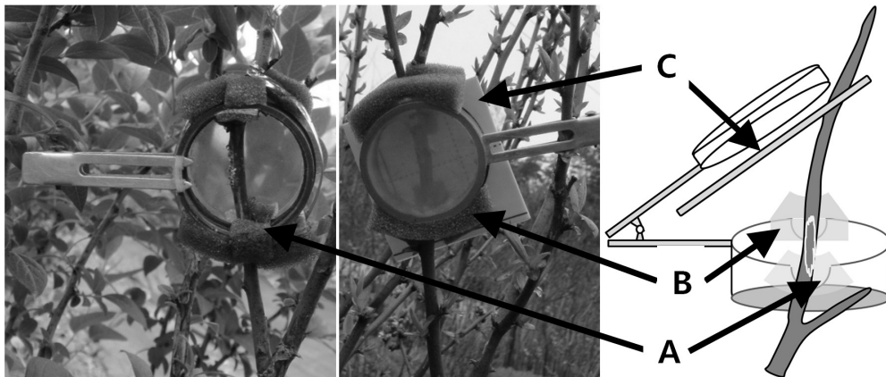
Fig. 1. Modified clip cage for investigating the emergence of Ricania sp. nymphs from overwintered egg mass on blueberry. A: Groove for twig, B: Sponge to block gaps between twig and groove, C: Sticky trap.
